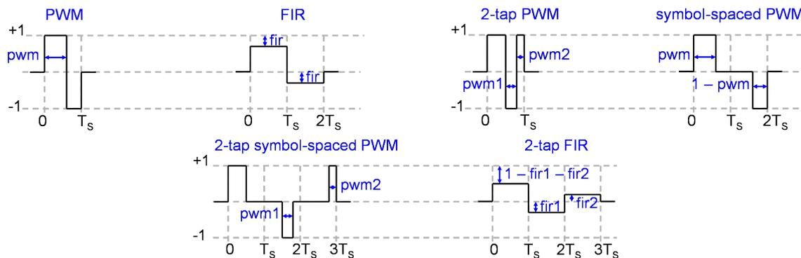
Figure 5. Equalization methods.
