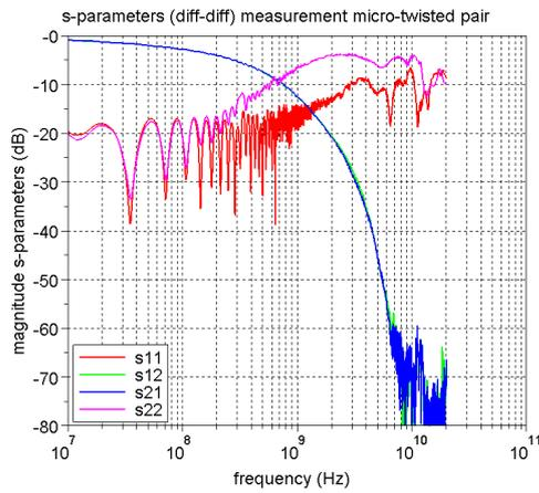
**Figure 1.** Measured s-parameters of 2.5m micro twisted-pair cable.
