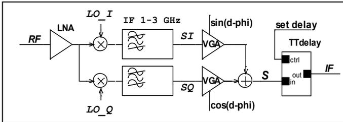
Fig.2. Front-end channel in RFIC1
