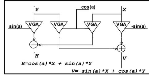
Fig.7 Vector modulator with VGA's
