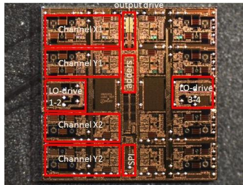
Fig.14 Chip photograph, die area is 3.8x4 mm
