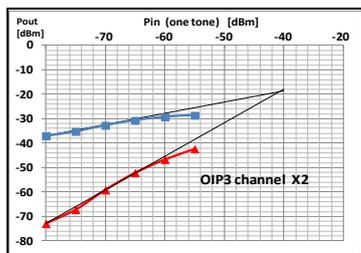
Fig.11 Measured OIP3 of channel X2
