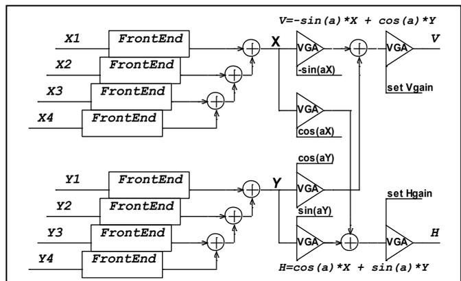
Fig.1. RFIC1: eight X/Y frontend-channels combined to 1 V/H output
