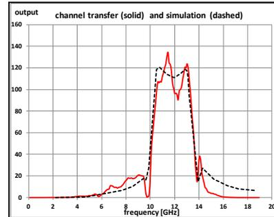
Fig.9 IF-transfer (linear scale) simulation (dash) and measurement (line)
