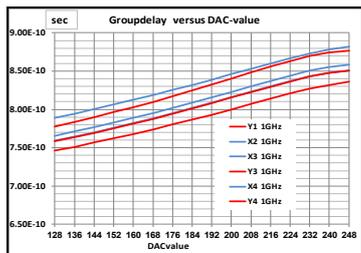
Fig.13 Measured max. TT-delay range versus DAC value
