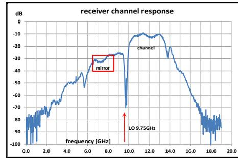
Fig.8 Measured overall channel response
