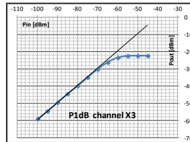
Fig.10 Measured 1dB compression point of channel X3
