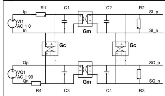
Fig.3. Differential second order active poly-phase BPF
