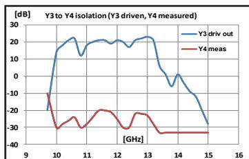
Fig.12 Measured channel to channel isolation
